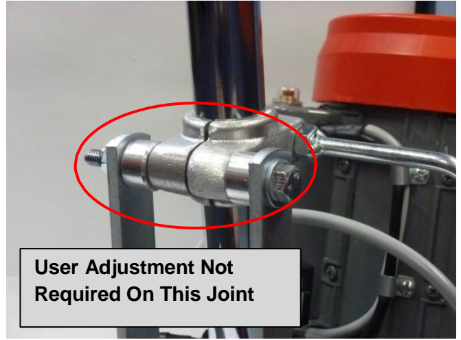
Pic 10 Factory Set Joint on Focus Suds Classic Models
