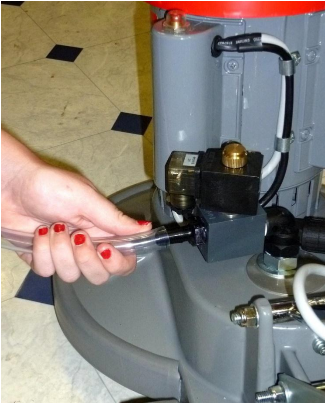
Pic 6 Attaching Hose to Solenoid Valve.
