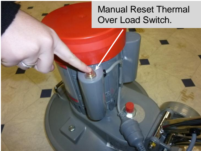
Pic 14 Motor Thermal Overload Switch
